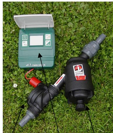
Magnetic valve, computer and filter
