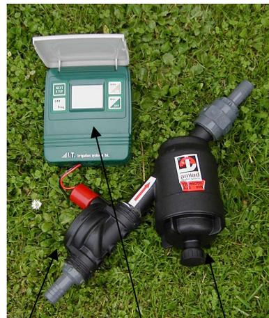
Magnetic valve, computer and filter
