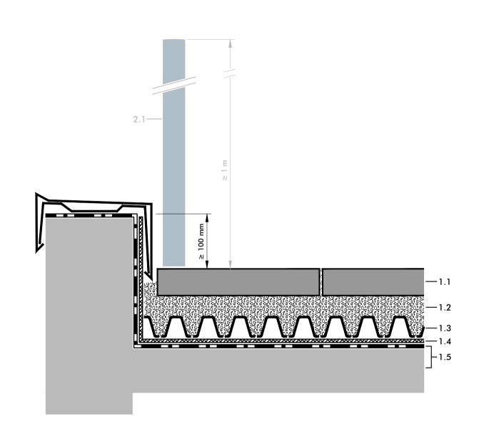
2.1 Guardrail Base GB with railing (see Guardrail Base detail)
