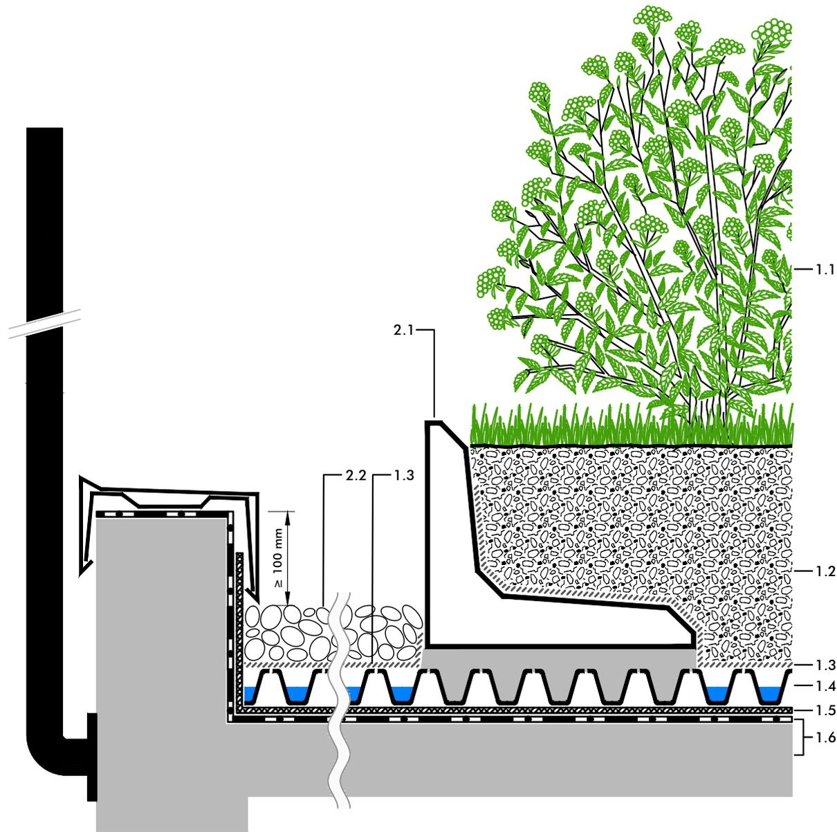
2.1 ZinCo Concrete Kerb in concrete foundation
