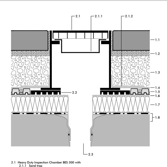
2.1.2 Filter sheet collar 2.2 Elastodrain<sup>®</sup> EL 202-Support Board
