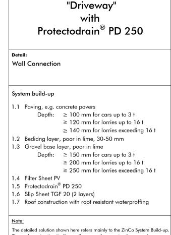
The roof construction itself as well as any other constructions are shown schematically and must be planned according to the relevant standards and guidelines.
