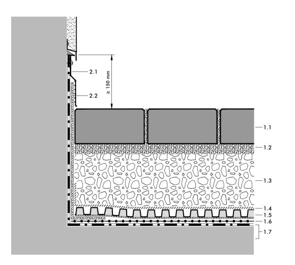
2.1 Clamping Profile AP 1502.2 Protection Mat Strip RS-M
